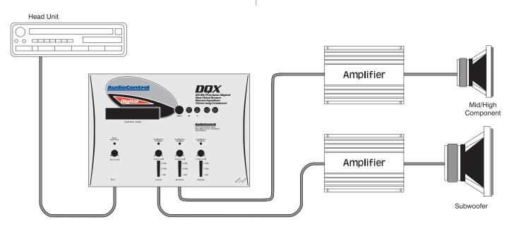
Figure 4: DQX in a two-way system
